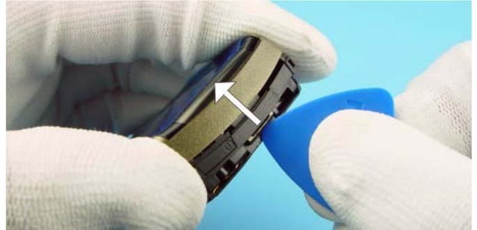
Unlock the top guidance to remove the A-Cover.
