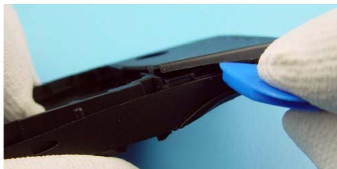
Unlock Antenna on both sides with SRT-6.
